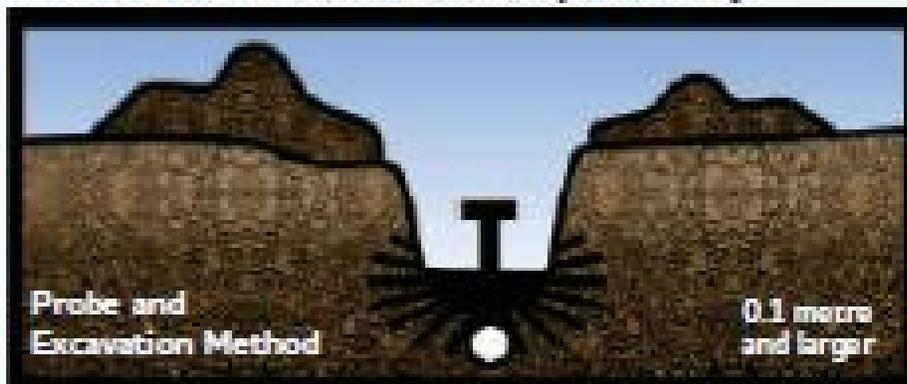
In addition to other excavation methods previously mentioned, a probe and excavate technique can be used for gas pipelines 0.1 metre and larger in diameter.
