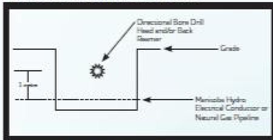
Drilling above a Manitoba Hydro electrical conductor or natural gas pipeline.
