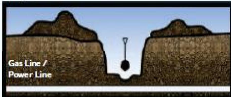
Dig a trench by hand across the full width of the excavation (perpendicular to or "across" the pipe). If the line is not uncovered, mechanically excavate to one half the depth of the trench. Repeat this process until the line is exposed.
